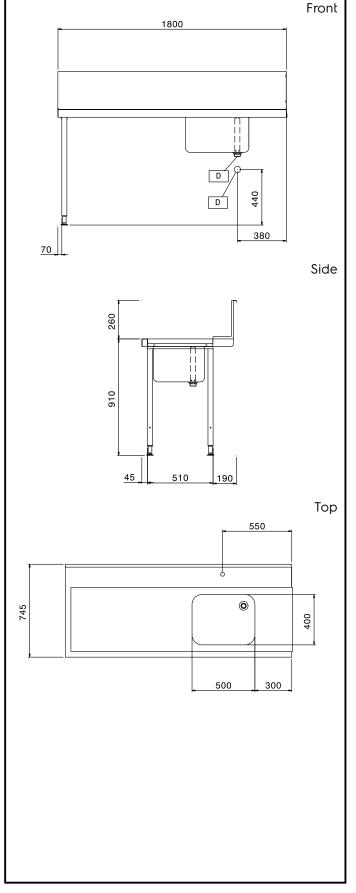
Handling System for Hood type Pre-wash Table with Bowl Left to Right, 1800mm
